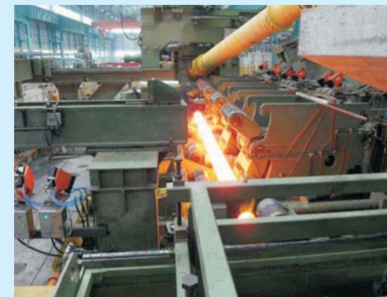
Seamless pipe hot-rolling mill Capacity: 200,000 MT/year
